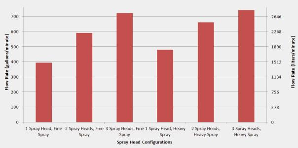
Total flow rates of different spray head configurations. The approximate total flow rates in gallons/minute (left vertical axis) and liters/minute (right vertical axis) of three possible spray head configurations. The "fine spray" opening is ¼ inches in height, and the "heavy spray opening" setting is ¾ inches in height. These flow rates were recorded on an MAC6 CAT730 with an M-3 Mega water pump.
